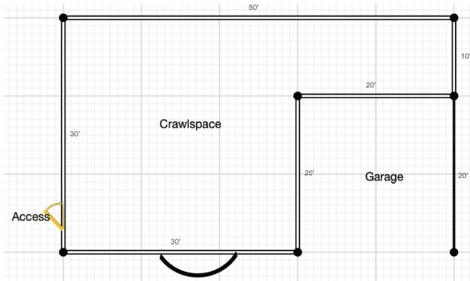
Step 1 - Calculate the amount of crawl space area that will need to be ventilated. In this case it's 1100 square feet. (length x width = area)
